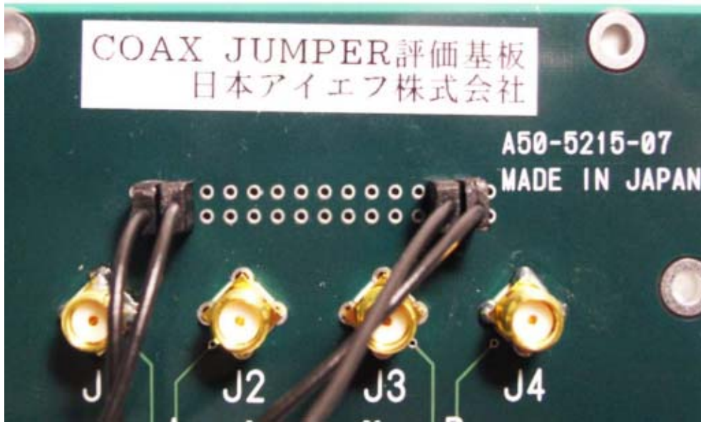
Picture-1 TDR / TDT Test Board Test Sample: Straight termination, AWG#28 L=500mm
